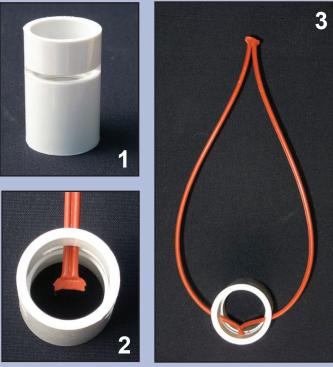
Insert CM/LR TT dispenser until it stops at notch in the middle of coupling. Spread dispenser the length of the cut in the coupling. Flip dispenser back overcoupling to lock in position. For information on how to make applicators and how to apply, visit our website or contact your local distributor.
